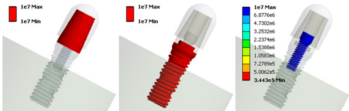
Figure 21. Fatigue Life Result for the BAM Implant with Maximum Load of 300 N Abutment (Left), Fixture (center) and Abutment Screw (Right)
