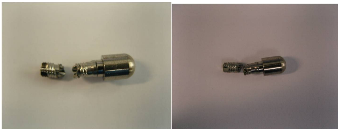
Figure 29. Fractured Implant from Fatigue Test with Maximum Load of 300 N Failed at 173,612 Cycle (Left) and Failed at 208,081 Cycle (Right)
